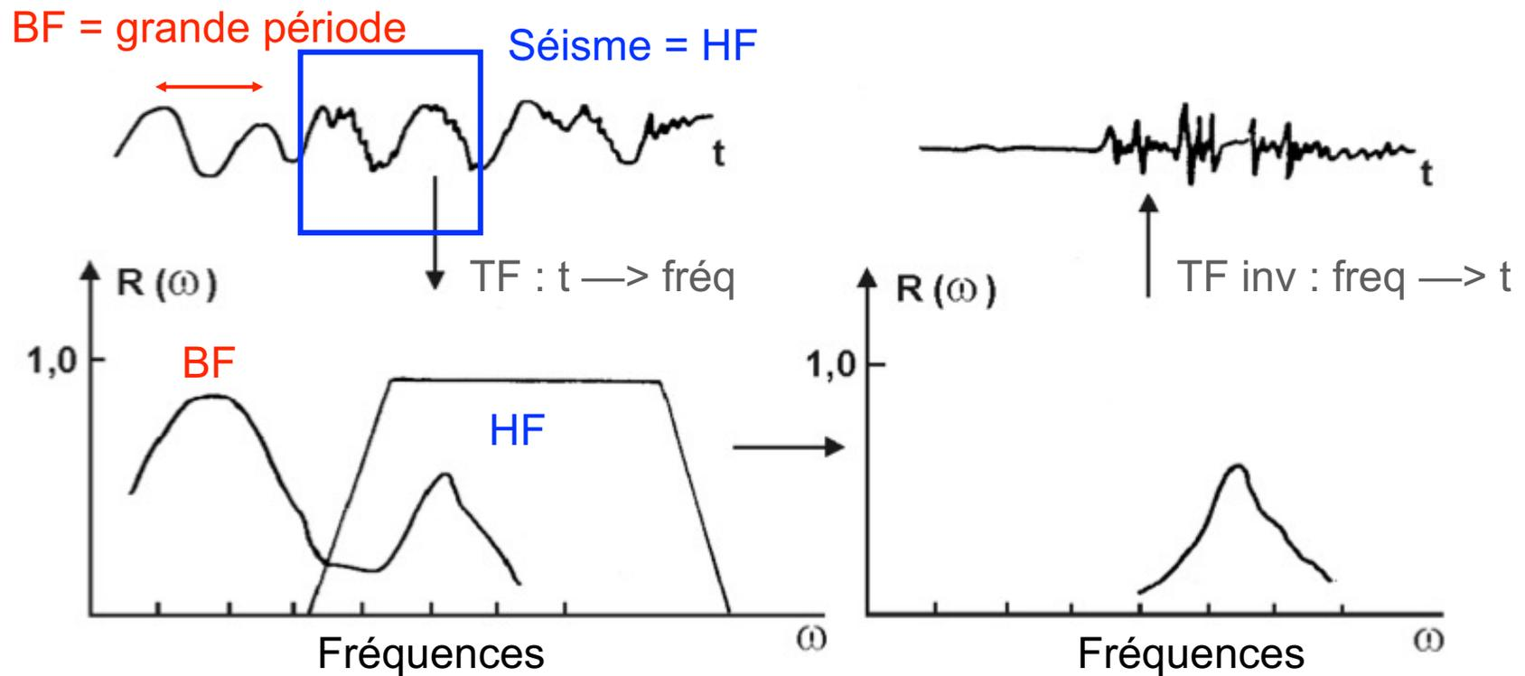
**Fig. 4.26** Principle of FOURIER transform and bandpass filtering of a seismic record.
