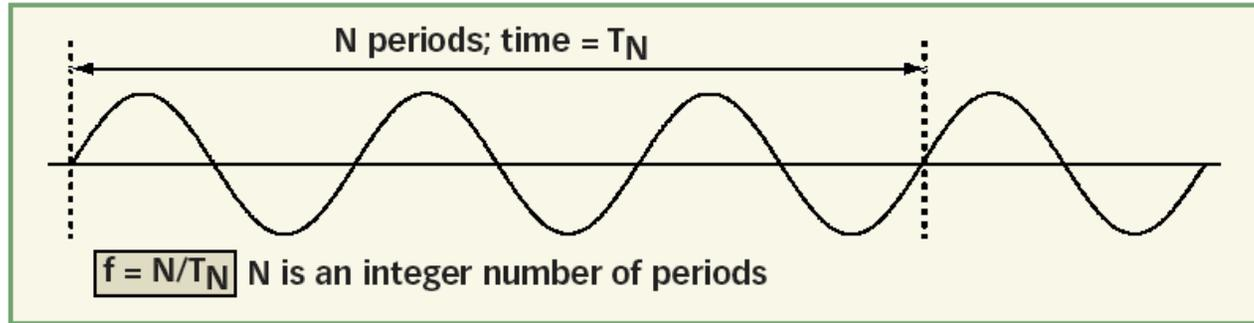
1. This graphical representation shows how a counter calculates frequency from a measurement of period time.
