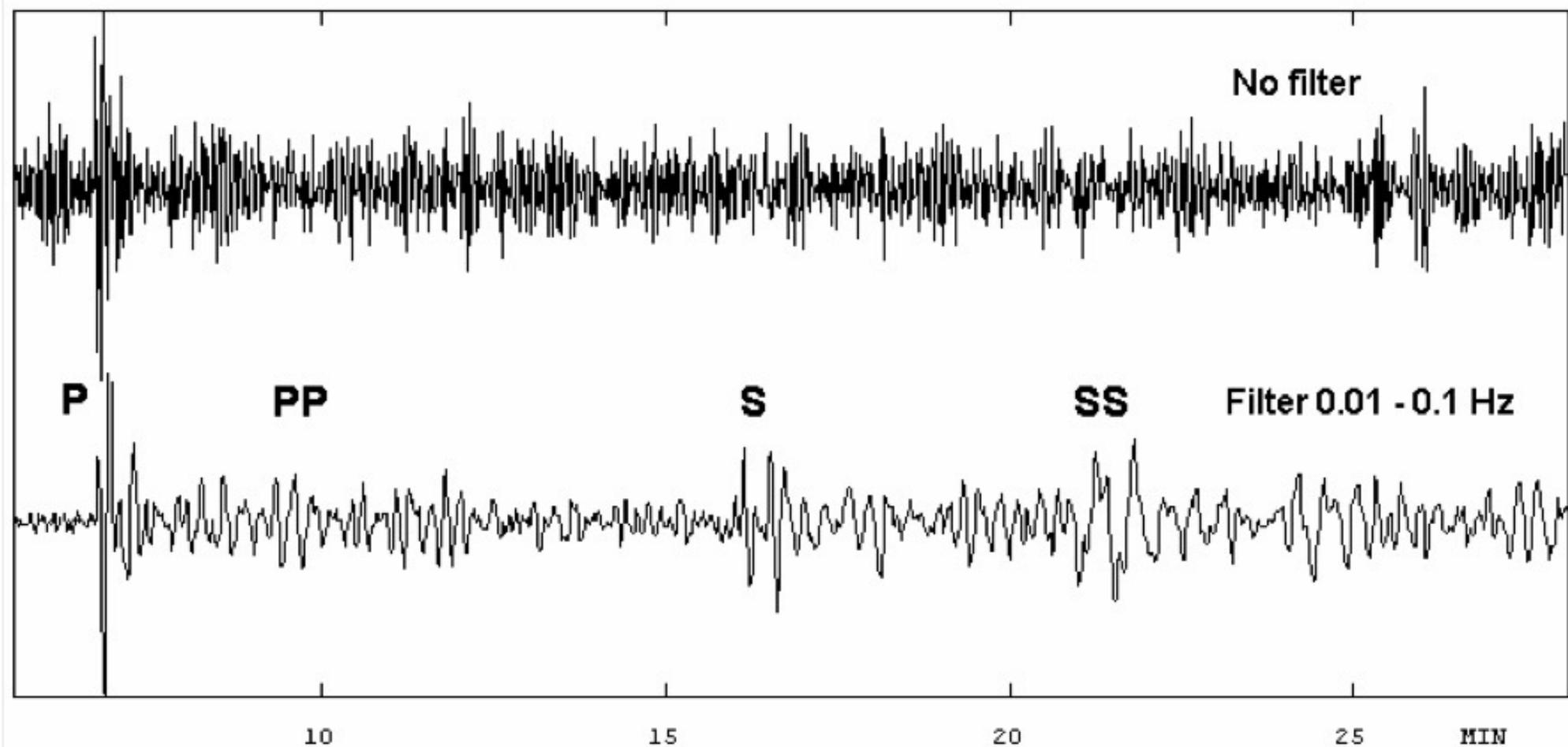
**Fig. 4.27** Recording of a LP trace at a broadband station. The LP trace has a flat velocity response from 360 s to 0.5 s. On the unfiltered trace (top), only the P-phase might be identified, while on the filtered trace (bottom), the signal-to-noise ratio is much improved and several later phases are clearly recognizable since the microseisms have been removed by filtering (courtesy of J. Havskov, 2001).
