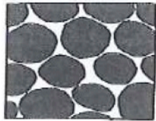
(a) high porosity — rounded grains, uniform size (good sorting)
