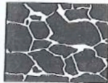
(d) very low porosity — angular grains, many sizes (poor sorting)
