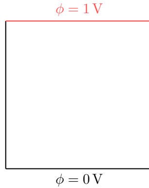
Figure 1: Electrostatic problem in vacuum to solve. An empty space is delimited by 4 conductors. Three of them (in black) are at zero potential, the last one (in pink) is at a potential of 1 volt.
