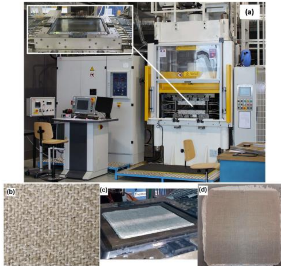
Fig. 1. (a) Fast induction-heated compression moulding press, (b) Close view of flax/PP commingled fabric, (c) 8 plies fabric layup and (d) Manufactured composite laminate.
