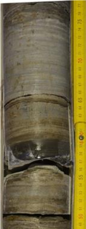
Figure 11: Banc d'anhydrite massive.
