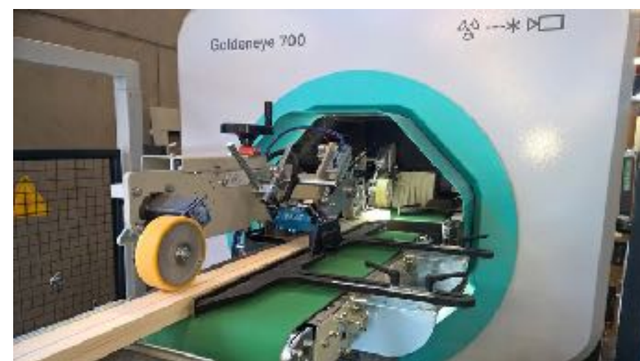
Scanner RX (GoldenEye, Microtech) ~7 m/s
